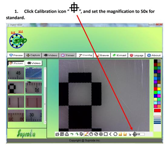
2. Put the Digital Viewer microscope on the Calibration Pattern sheet, you can see the black/white block on the screen.
